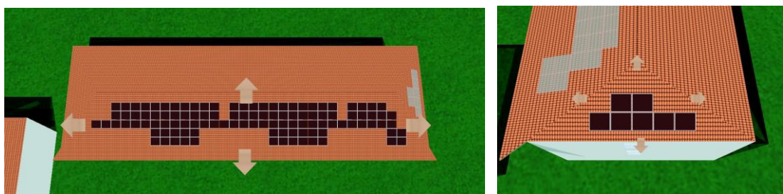
Fig. 5.31. Solar cell panels layout (Pictures done with PV*SOL Expert Pro 5.5, © Valentin Software [1] )
