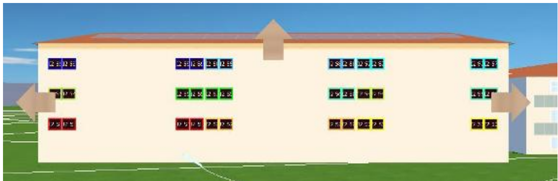
Fig. 5.14. PV strings layout on Balconies House Q (Picture done with PV*SOL Expert Pro 5.5, © Valentin Software [8] )
