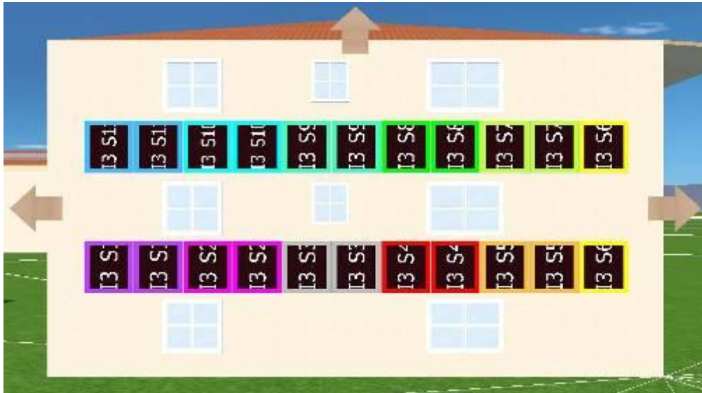
Fig. 5.20. PV strings layout on Facade House N (Picture done with PV*SOL Expert Pro 5.5, © Valentin Software [8] )
