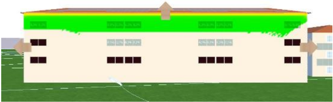
Fig. 5.13. Solar cell panels on Balconies House Q showing the shading effect (Picture done with PV*SOL Expert Pro 5.5, © Valentin Software [8] )
