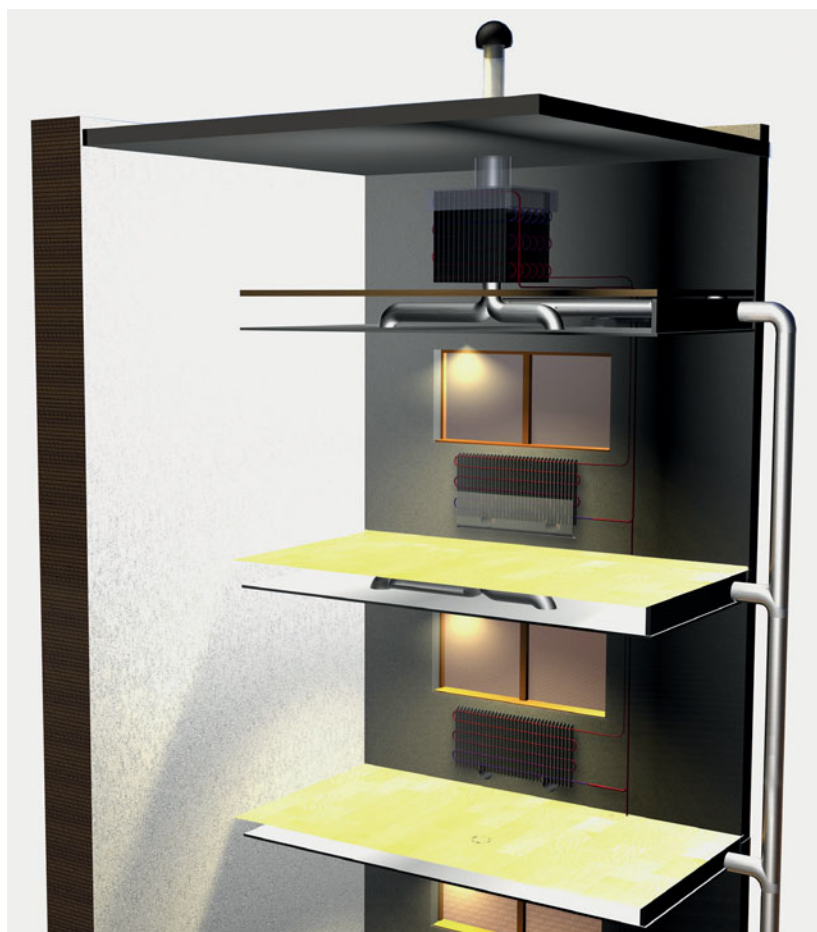
Façade-integrated natural ventilation system with heat recovery
